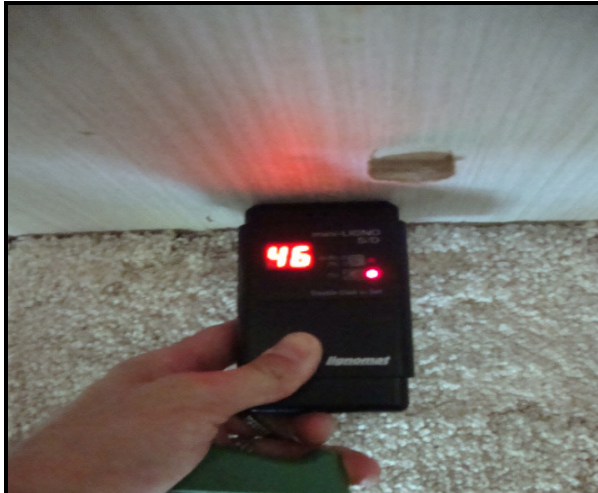
Elevated moisture in wall at SE corner of master bedroom (page 4, A).
